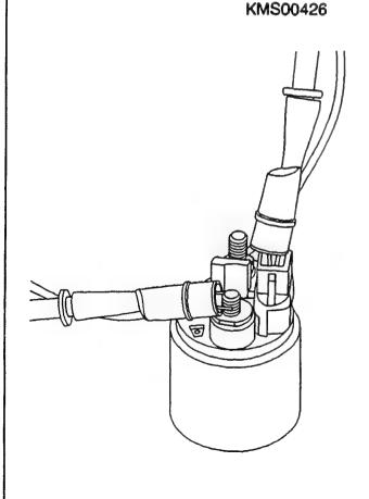
Checking solenoid switch
